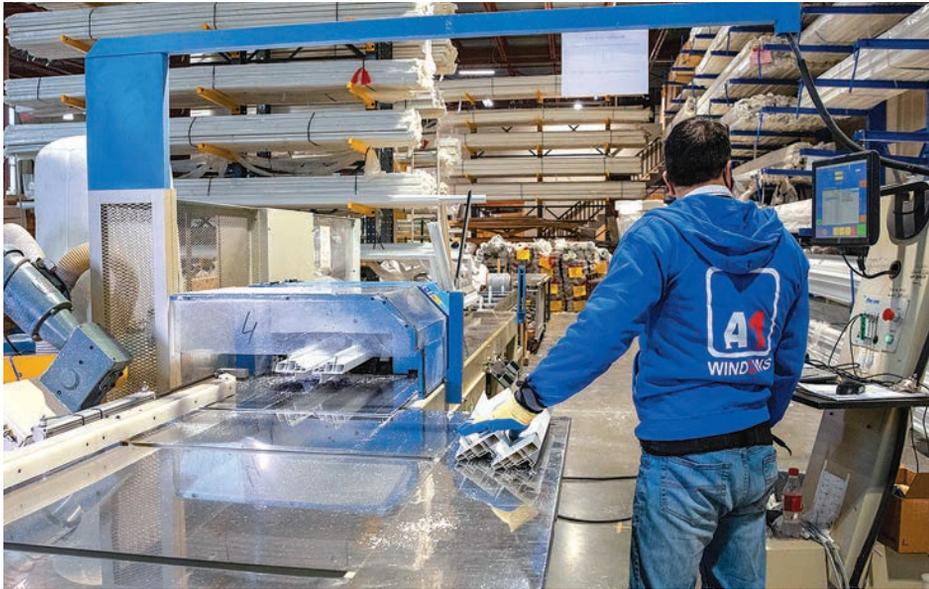
*Cutting on the Pro Line CNC automated cutting saw.*
